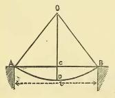
Let ADB be the beam loaded in the centre with a load w. Let AB = l and  $\theta$  the angle of deflection. The reactions at Aand B will be at right angles to the inclination of the beam at these points, and may be represented by the lines AO BO. Producing the strain in the beam at the point D there is :— 1st, the vertical component of the reaction at the abutments multiplied by the distance at which the force acts—viz.,
